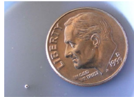
Size comparison of mercury found in a typical compact fluorescent light bulb sold in the U.S. Photo courtesy of Monte Helm, Ph.D. Fort Lewis College
