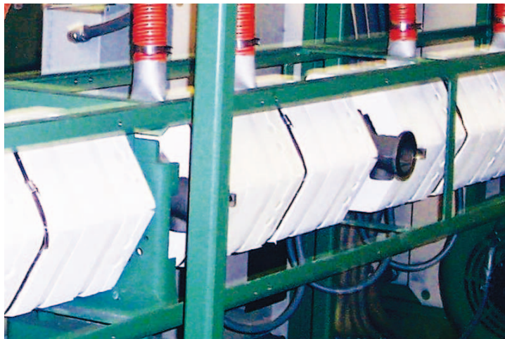
REX TCS™ installed on extruder barrel at Pactiv Corporation
