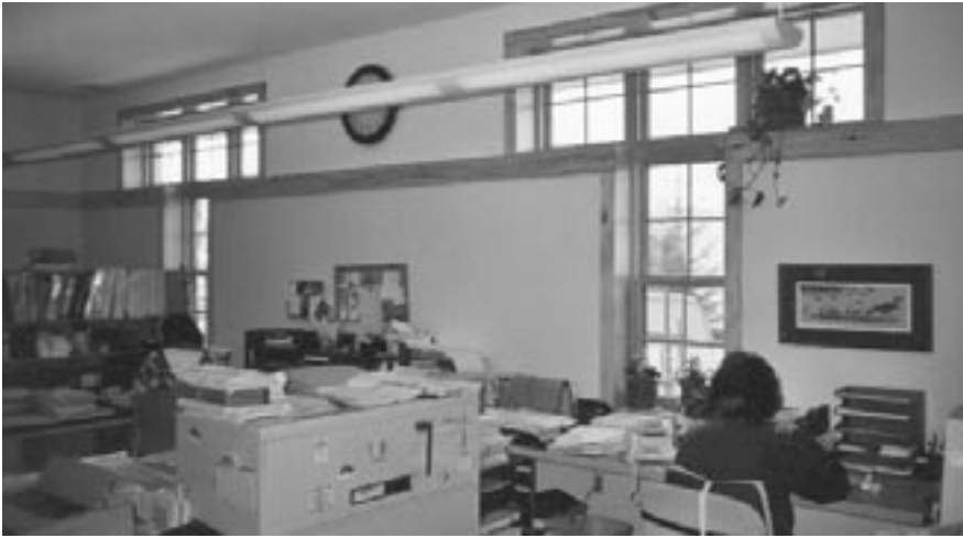
(above left) T-shaped windows on the south side of the building increase the general light level in the office while reducing glare on computer screens.
