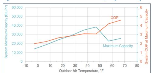
Figure 2. Illustration of ducted ASHP COP and capacity variance by outdoor air temp.
