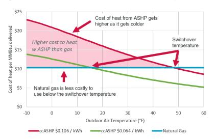
Figure 3. Illustration of impact of switchover temperature on operating costs.
